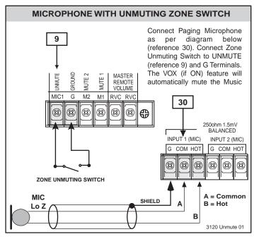
Fig. 18 - Microphone and Zone Unmuting Diagram
